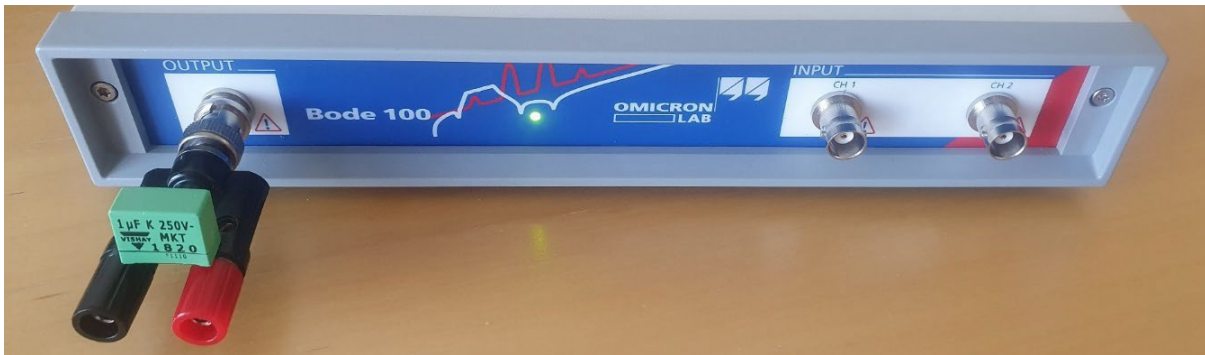
Figure 14: One-Port -BNCアダプターへ接続
